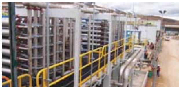
Mine waters are notoriously tough to treat because of the volume and the complexity of the waste streams. HW Process Technologies installed and operates the largest membrane treatment system in the global mining industry. This unit treats millions of gallons per day, while reclaiming tons of usable metals and chemicals from the waste stream at this site in South America.
